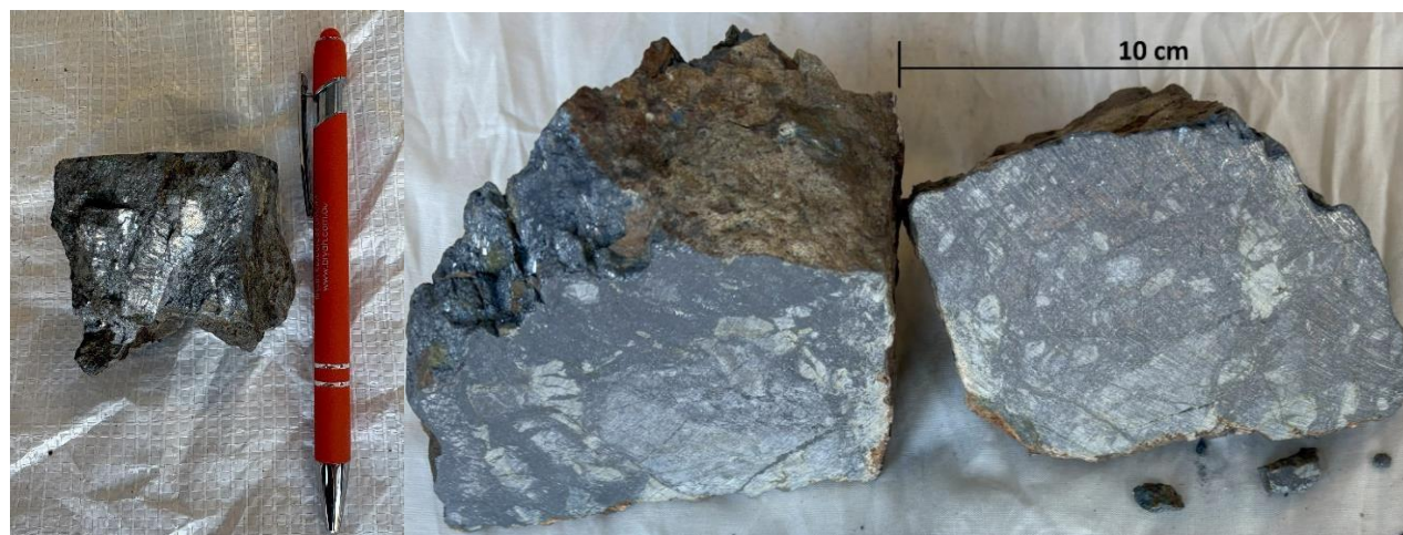
Archive rock chip specimen from BBD02507 with a stibnite crystal approximately 4cm long (left) And for archive rock chip specimen from BBD02506 with brecciation texture (right)
