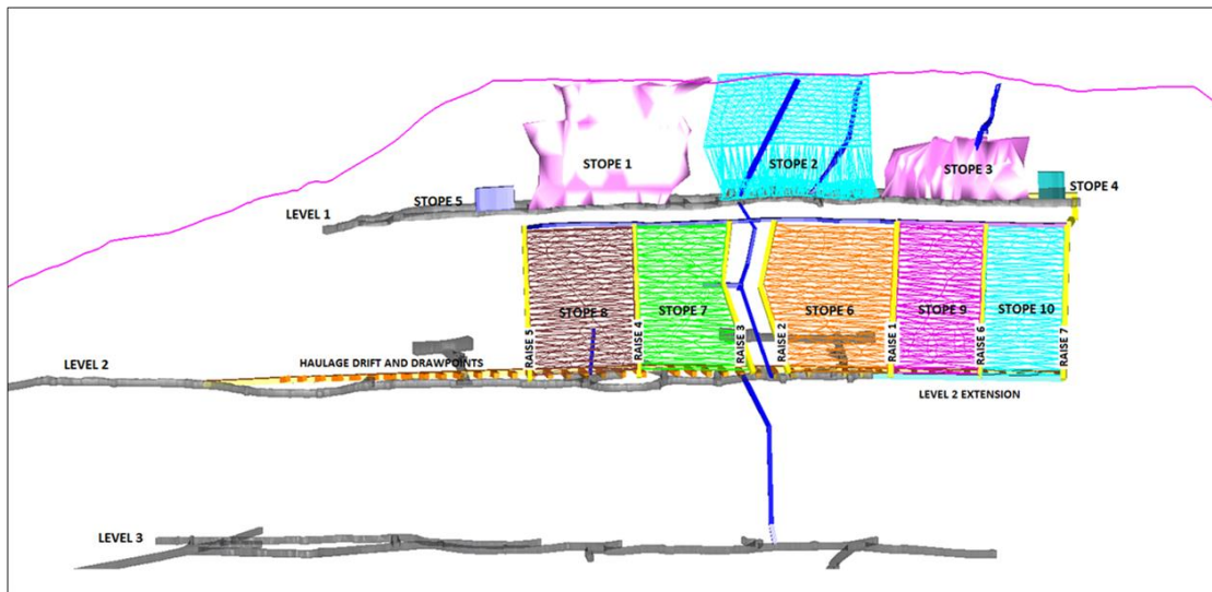
Figure 3: Section view of the Treasure Mountain underground workings (Level 1, 2, 3 with stope projections)
